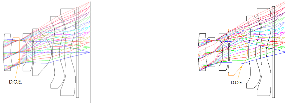
(a) DOE is at the rear surface of the 2nd lens (S4)
