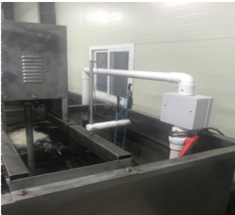
Fig. 10 Seaweed Mixture Concentration Sensor Operation
