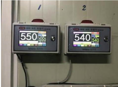
Fig. 9 Seaweed mixture concentration control display and remote control device
