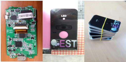
Fig. 4 Location tracking module
