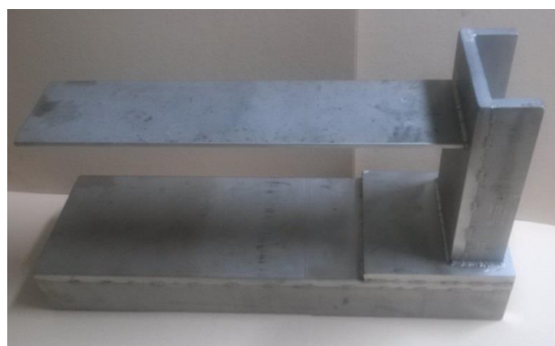
Fig. 11 Load cell structure of cantilever beam type subjected to end vertical downward Load
