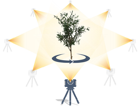
Fig. 2. Schematic to Show the 3D Scan Setup
