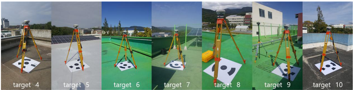
Fig. 2. GNSS static survey of check points
