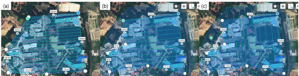
Fig. 4. Flight routes: (a) method 1 (vertical 1), (b) method 2 (vertical 2), and (c) method 2 (oblique from north to south)
