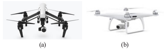
Fig. 3. Data acquisition equipment (a) inspire 1 (b) phantom 4 pro
