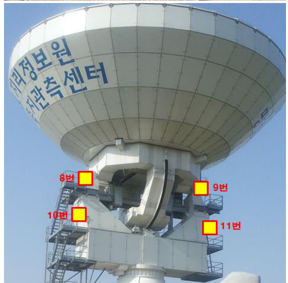
Fig. 4. Location of reflective targets for co-location survey (NGII, 2019a)
