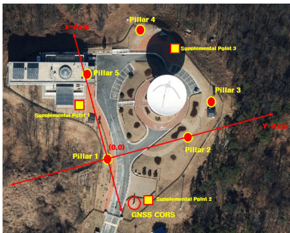
Fig. 3. Location map of Sejong VLBI station and pillars used for co-location survey (NGII,2019a)
