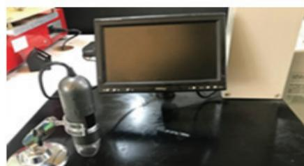
Fig. 6. USB microscope used for scaffold pore shape photograph.
