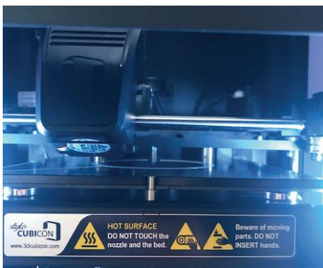
**Fig. 9.** Scaffold printing using FDM 3d printer.
