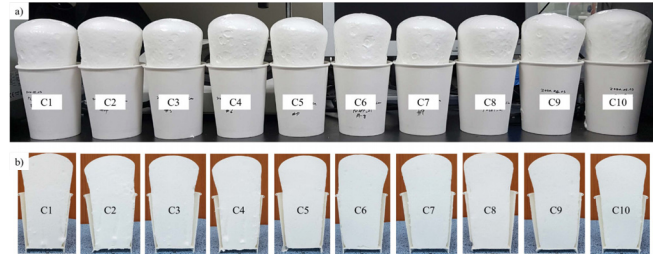
Figure 6. The frontal view of polyurethane foams with the same time duration (10 min) between the gelling and blowing reactions. (a) for the frontal view (b) for the cross-sectional view.
