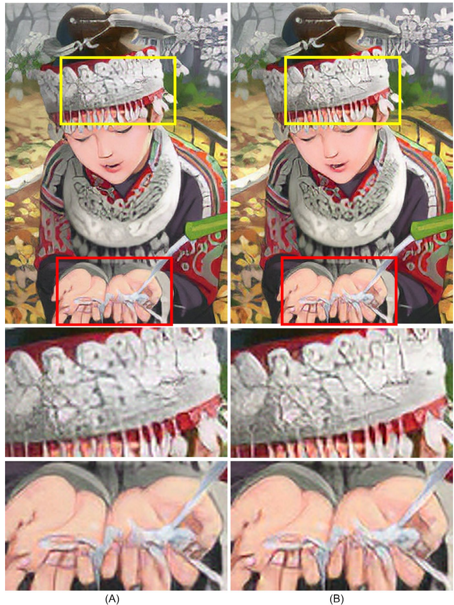
FIGURE 6 Comparison between SRGAN_{VGG} and cSRGAN at the similar objective image quality for the upsampling factor of 4 on Set14: (A) Result of SRGAN_{VGG} (PSNR: 21.67 dB); and (B) Result of cSRGAN (PSNR: 21.56 dB). For each test image, the second and third rows are the image patches corresponding to the yellow and red rectangles in the top row. These are best viewed with zoom
