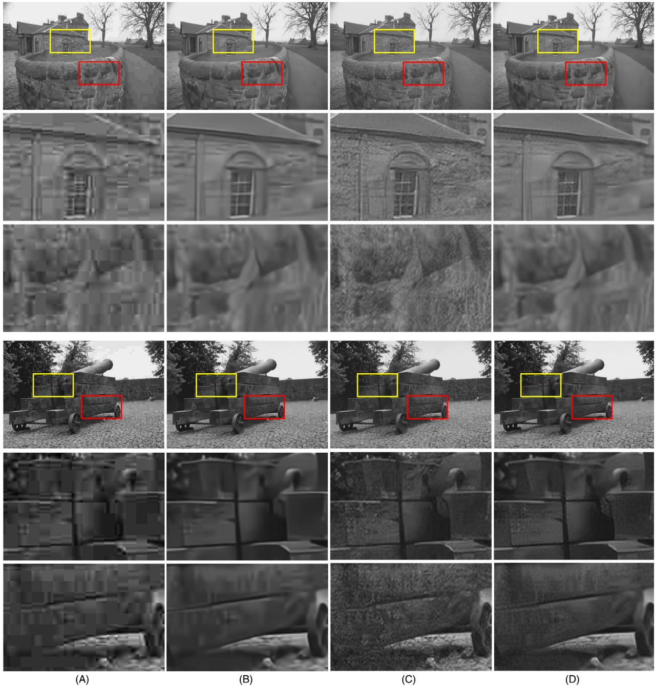
FIGURE 2 Comparison of different ARGAN training schemes under quality factor 10 on BSDS500: (A) JPEG (PSNR: 26.09 dB (top), 25.09 dB (bottom)); (B) ARGAN base (PSNR: 27.48 dB, 26.18 dB); (C) ARGAN VGG (PSNR: 25.32 dB, 23.67 dB); and (D) cARGAN (PSNR: 27.21 dB, 25.86 dB). For each test image, the second and third rows are the image patches corresponding to the yellow and red rectangles in the top row. These are best viewed with zoom
