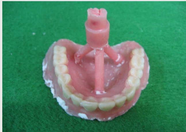
Fig. 6. Denture base with 3-forked sprues (Mak Press).
