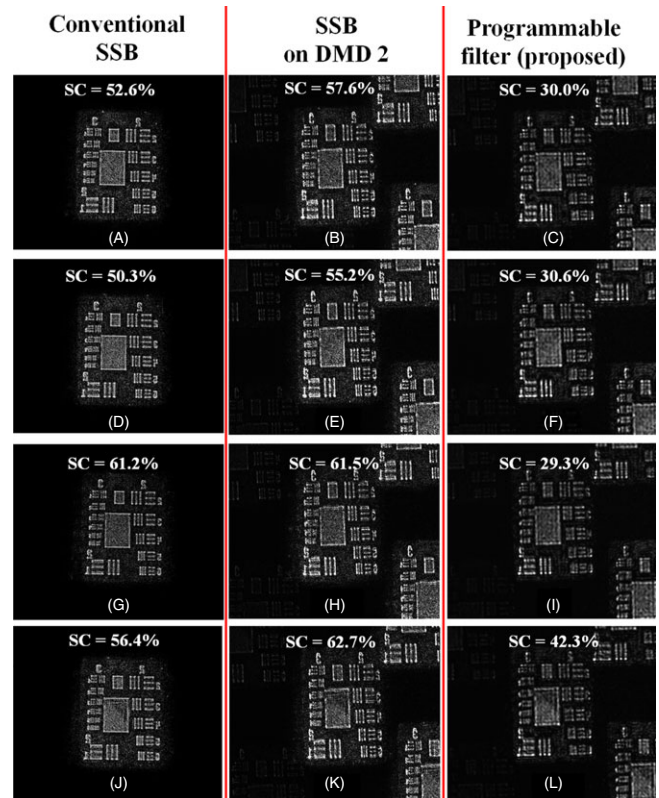
FIGURE 9 (A), (B), and (C) are the reconstructed hologram images of the CGH in Fig. 8(A). (D), (E), and (F) are the reconstructed hologram images of the CGH in Figure 8(C). (G), (H), and (I) are the reconstructed hologram images of the CGH in Figure 8(E). (J), (K), and (L) are the reconstructed hologram images of the CGH in Figure 8(G)
