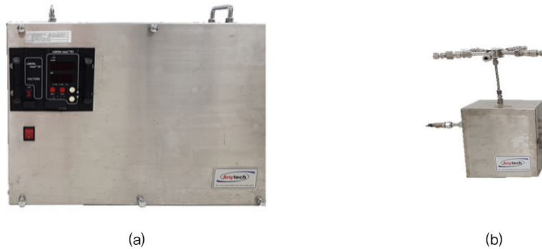
Fig. 3 Equipment for sensory evaluation (a) generator of clean air, (b) 5-way distributor
