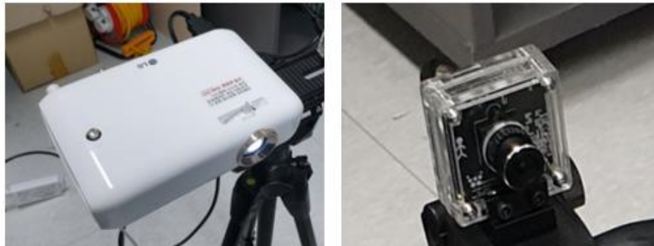
Figure 2. PH550 DLP Projectors (a), oCam-5CRO-U (b)
