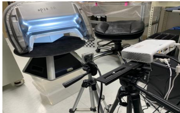
Figure 9. Structure of car press parts 3D scanning by optical method
