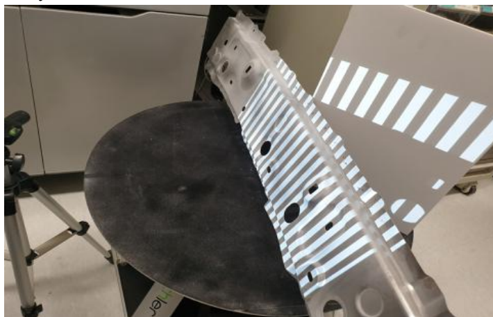
Figure 13. 3D Scanning of Press Parts of a Real Vehicle Using the Proposed Method
