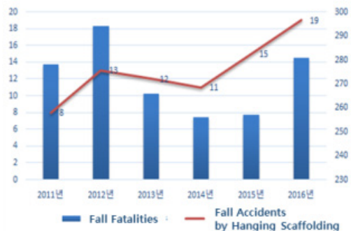
Fig. 1. Hanging Scaffolding Disaster Status
