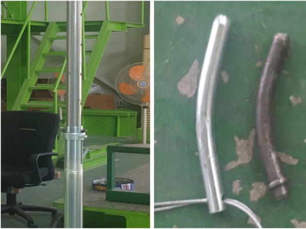
Fig. 5. Compressive test and support pins(pipe support).
