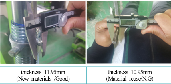
Fig. 6. Measuring thickness support pins.
