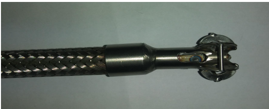
Fig. 5 Improved soot measurement probe
