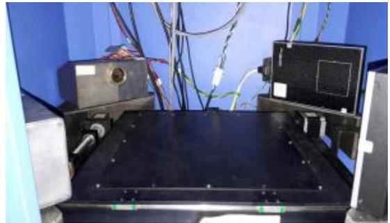
Fig. 1 X-ray generator and detector
