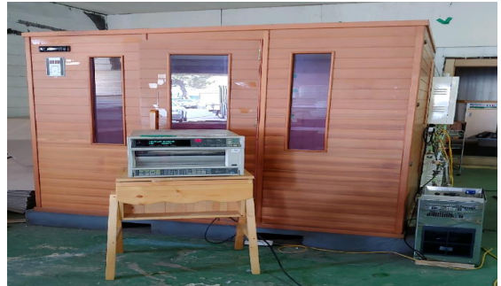
Fig. 1 Cooling system using cold water panels in small building walls
