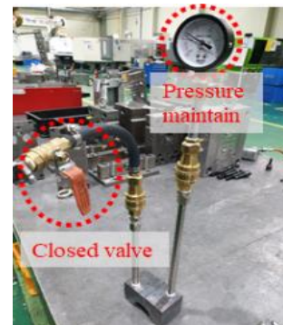
Fig. 11 Air leakage test of the test mold core
