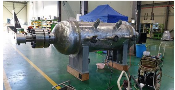
Fig. 9 Hydraulic pressure test
