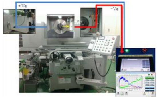
Fig. 2 ELID Grinding system for experiments
