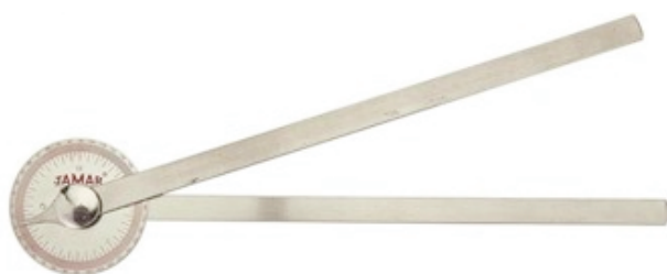
Fig. 7. Stainless steel goniometer (JAMAR stainless steel 360° 14 inch goniometer, Greendale, Wisconsin, USA)
