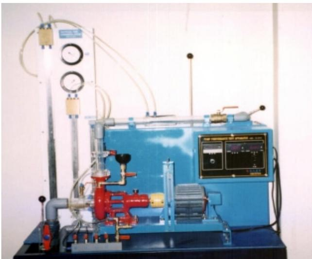
Figure 1. Experimental apparatus of centrifugal pump.
