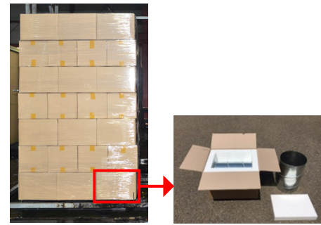
CEP dummy of combustibles CEP unit combustible Figure 2. Cartoned expanded plastic (CEP) combustibles.
