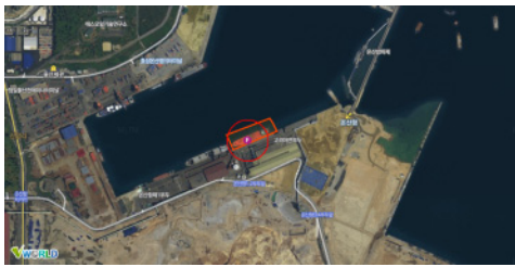
Figure 7. Influence range of the toxicity damage of benzene according to leakage time (Alternative scenario IV).
