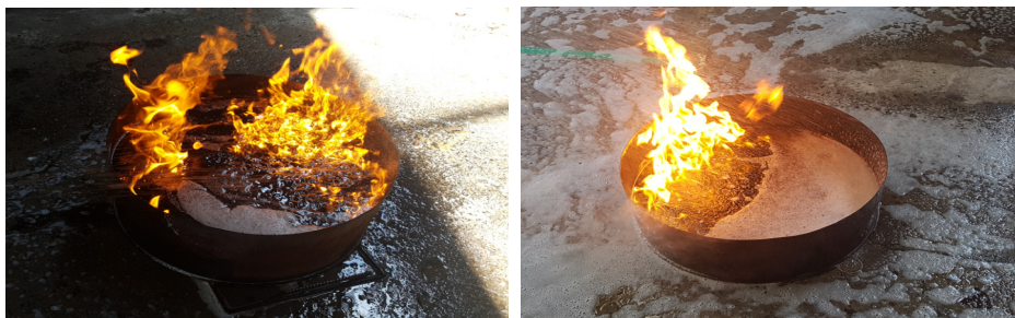
Figure 8. Foam blanket status of low-capacity radiation (left) and high-capacity radiation (right).
