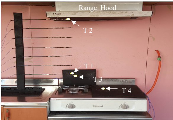
Figure 7. Device to measure ambient temperature change due to the pot overheating.
