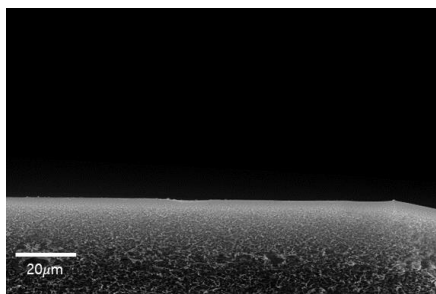
Fig. 2. Scanning electron microscopy (SEM) image of neat polysulfone support.
