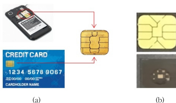
Fig. 2. Smart chip card used in public. (a) Smart chip cards are embedded in mobile phone, credit card, etc. in public. It has some characteristics that easy to extract in case of radiation accident to measurement radiation dose and simple preparation process to experiment. (b) The uv epoxy resin of back side of smart chip cards reacts to radiation dose and light. Thus it can be used to measurement of radiation dose and reconstruction of radiation.
