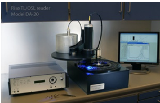
Fig. 3. Radiation dose measurements reader (Risoe TL/OSL-DA-20 TL / OSL). After irradiation, the dose of radiation to sample are measured by this reader using built-in blue light source.
