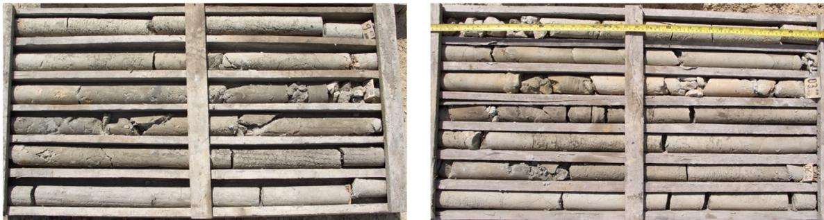
**Fig. 6.** The drilling core of the Roto South area in KIDECO
