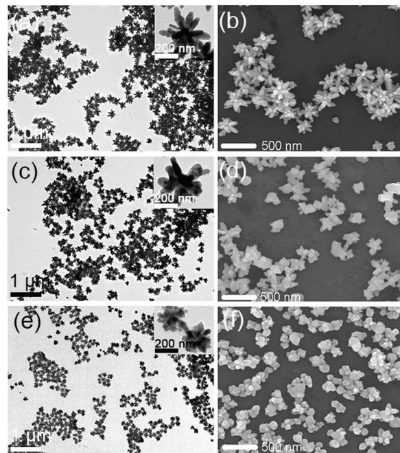
**Fig. 1.** TEM and SEM images of sample 1 (a, b), sample 2 (c, d), sample 3 (e, f) with urchin Ag NPs.
