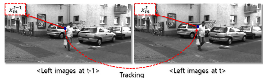
Fig. 5. Feature Tracking using KLT Tracker[5]
