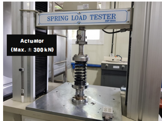
Fig. 6. Setup for stiffness measurement of spring
