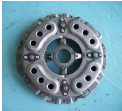
Fig. 7. Improved clutch cover including center ring
