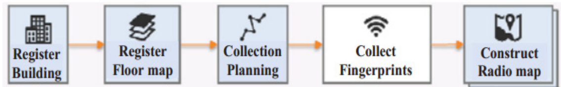
<Fig. 2> Collection Procedure of the Indoor and Radio Map
