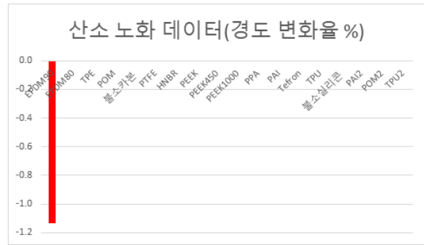
Fig. 8. Rate of Variation Hardness of Rubber Material
