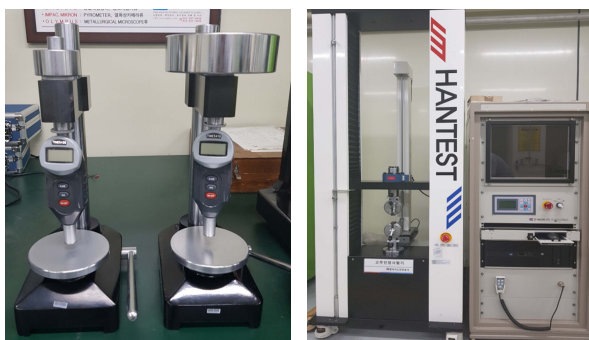
Fig. 3. Shore Durometer & Universal Testing Machine
