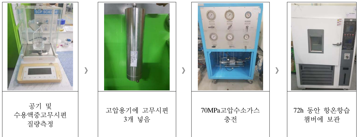
Fig. 2. Hydrogen Soakage Test
