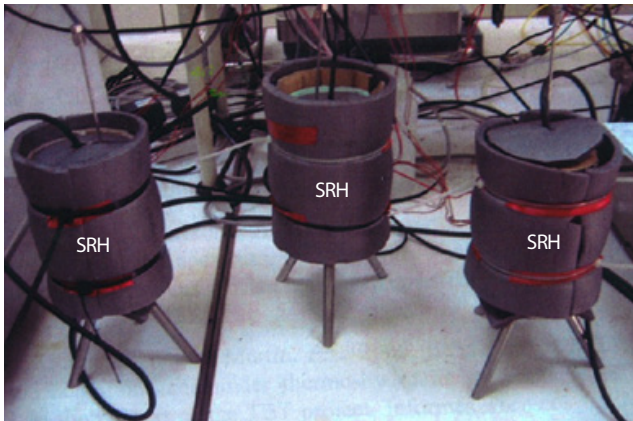
Fig. 6. Schematic diagram of the suction-measuring device of the RH-Cell/Sensor technique with silicone-rubber heater (SRH) [11].
