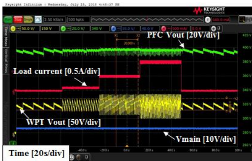
Fig. 17. Load regulation in standby mode.
