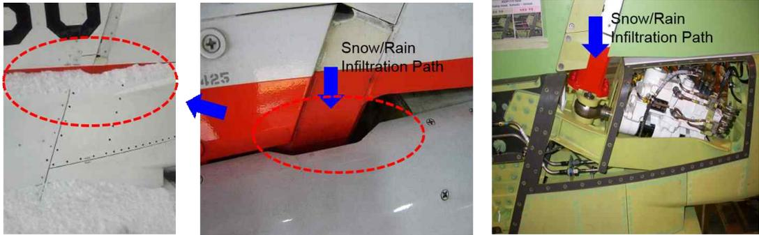
Figure 9. Water Infiltration Path to the FCISA
