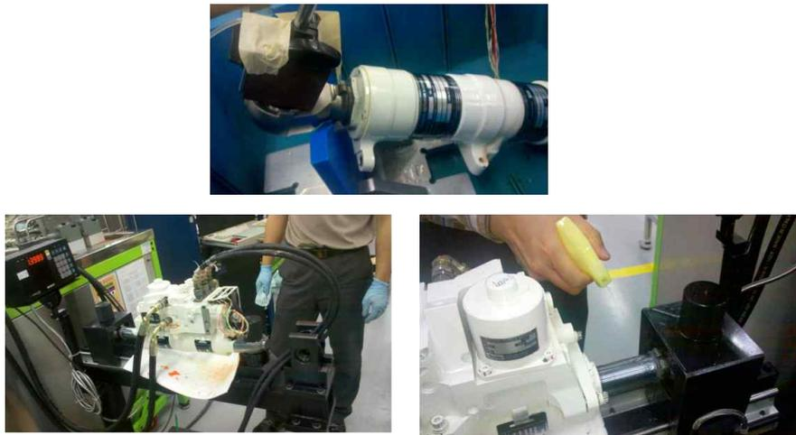
Figure 12. Simulation Test for Water Infiltration
