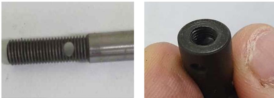
(a) Thread of a screw for firing pin (b) Thread of a screw for latch inside
