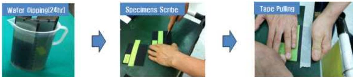
Figure 13. Wet Tape Test
