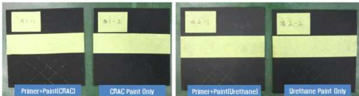
Figure 14. Specimens of Paint Adhesion Test
