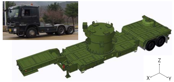
Fig. 1. Configuration of the trailer with dummy weight and tractor which used in driving tests
