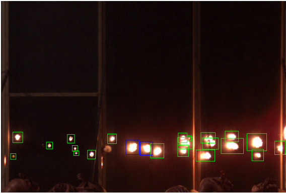
Fig. 3. An example of a captured AFT image with the AFT experiment setup illustrated in Fig. 2. Green: First penetrating fragments. Blue: Growing fire after the first penetrating fragments
