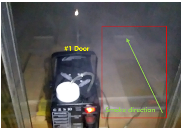
Figure 8. Smoke pattern observed while the door is open
