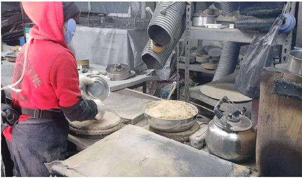
Figure 1. Cleaning stainless steel containers using diatomaceous earth powder
