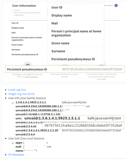
Fig. 3 Attributes sent by an identity provider (up) and received by the SAML4J example app. (down)
