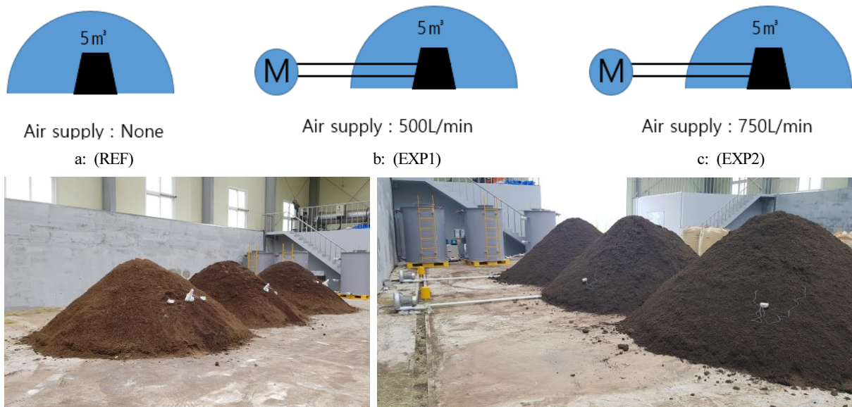
Fig. 2. Composting testing of swine manure.
