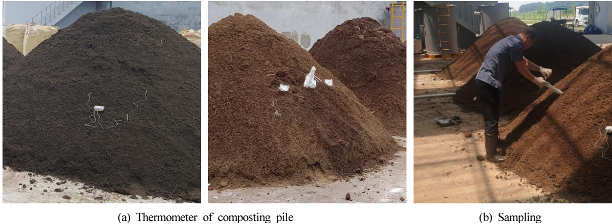
Fig. 3. Installment of temperature sensor and sampling of compost.
