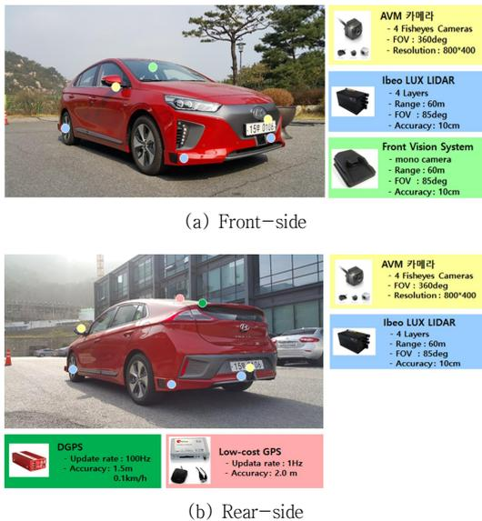
Fig. 1 Vehicle and Sensors configuration
